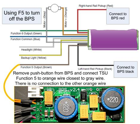
By default, the BPS orange colored wires labeled "SDN" are connected to a momentary contact push-button switch for manually initiated turn-off. Removing the push-button switch and
