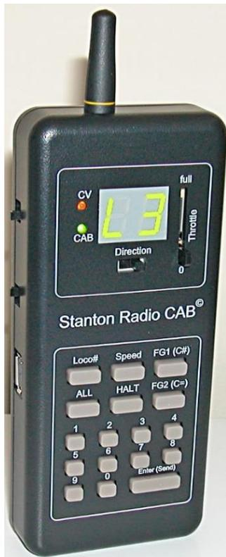
The throttle's number keypad is used to send a variety of commands, with actions determined by the task to which the keypad is assigned. Buttons labeled 'Speed', 'FG1' and 'FG2' assign the keypad to either speed step control or one of two function groups. Once assigned, the keypad continues this assignment until reassigned.
