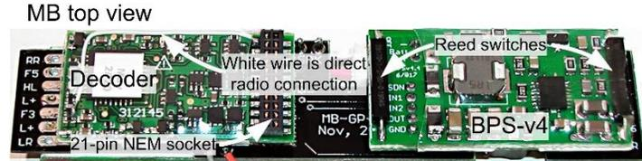
Lights and, if using a sound decoder, a speaker must be installed somewhere in the loco. If a battery does not fit, consider attaching a trailing "battery" vehicle. The MB includes current limiting resistors for all LED light outputs (headlight, rear light, functions F3, F5 and F6). Function F4 is used as a battery-off command.
