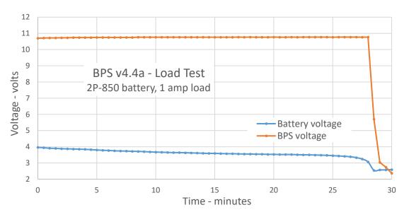
Battery voltage was 2.54 volts when BPS dropped output voltage. With resistive load, current continued to flow at a much lower level and graph shows a slight transient recovery of battery voltage. BPS ultimately shut down at approximately 2.5 volts.
