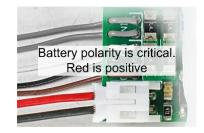
BPS-Lite is delivered with battery positive lead insulated. Since a voltage transient associated with plugging in the battery may turn on battery output, be sure to keep battery + terminal insulated until connections have been completed.
