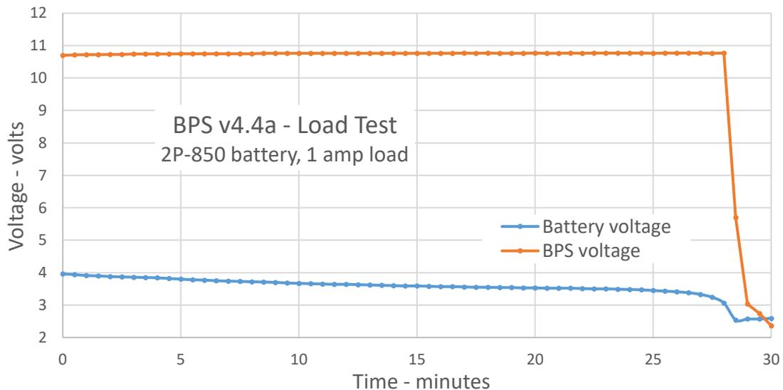
Battery voltage was 2.54 volts when BPS dropped output voltage. With resistive load, current continued to flow at a much lower level and graph shows a slight transient recovery of battery voltage. BPS ultimately shut down at approximately 2.5 volts.
