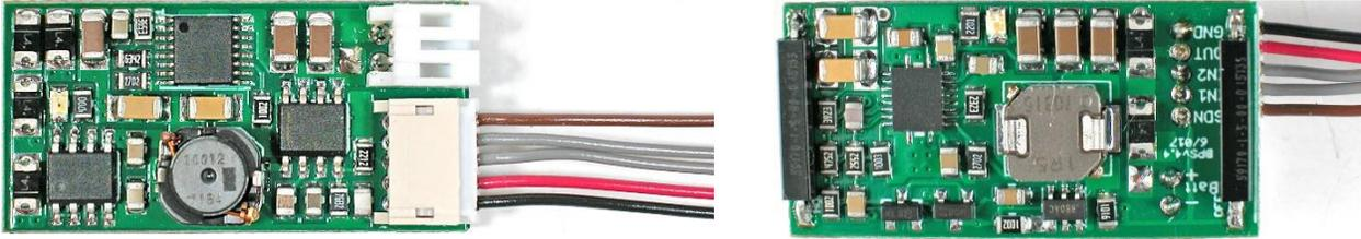
This fourth generation BPS battery power supply is intended for applications requiring up to 1 amp from a small package. Conceptually, there is no change from previous designs. Energy is provided by one or more lithium polymer (LiPo) cells connected in parallel and higher voltage output is produced electronically using a step-up converter. Battery charging, protection and switching are included within the design.
