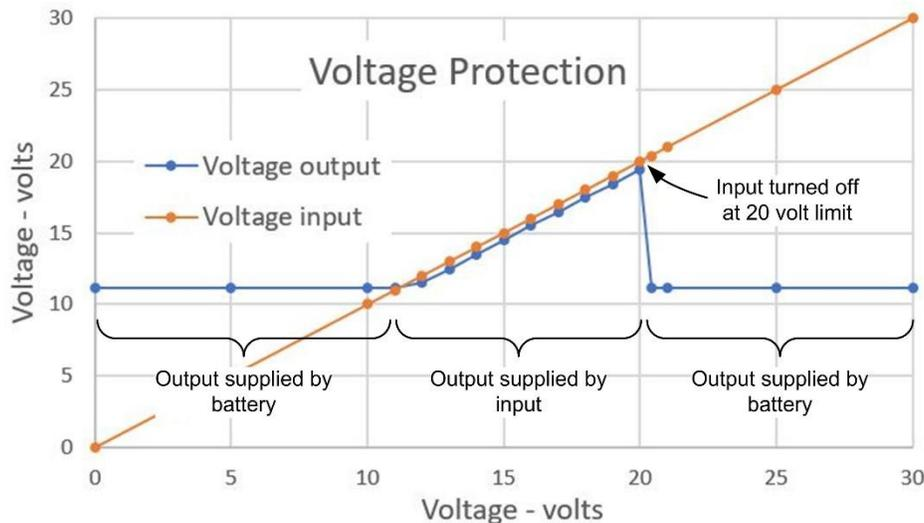
Most decoders can handle input voltage up to 20 volts, but best performance requires track voltage between 11 and 13 volts. Otherwise, there will be noticeable speed variations as BPS output switches between battery and track power.
